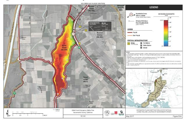
Figure 5-6 RD 349 – Estimated Flood Depth from Levee Breach Scenario
