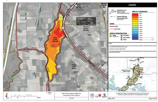
Figure 5-5 RD 349 – Time to One Foot Inundation after Levee Breach
