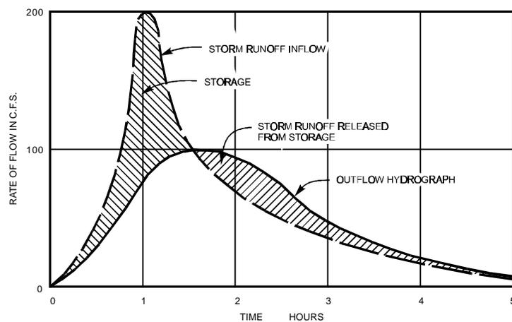
EFFECT OF ON-CHANNEL RESERVOIR ON STORM RUNOFF HYDROGRAPH
