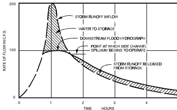
EFFECT OF OFF-CHANNEL RESERVOIR ON STORM RUNOFF HYDROGRAPH
