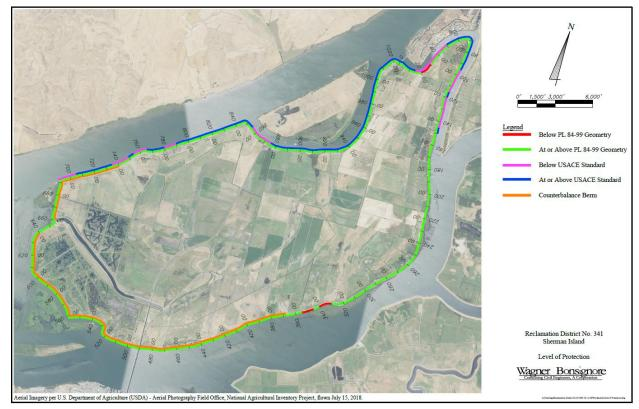
Figure 4-3 Level of Levee Flood Protection in Reclamation District 341
