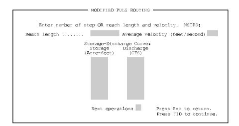
If the number of steps (NSTPS) is not entered, it is calculated from reach length and velocity with the following equation:
