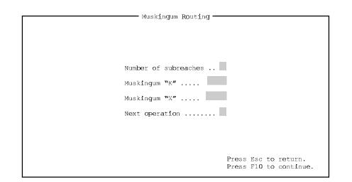
The number of subreaches is chosen to satisfy a stability criteria as described in the HEC-1 manual. The Muskingum "K" value may be approximated as the travel time in hours for the reach based on the flow velocity at normal depth. Typical ranges for the Muskingum "X" value are given below:
