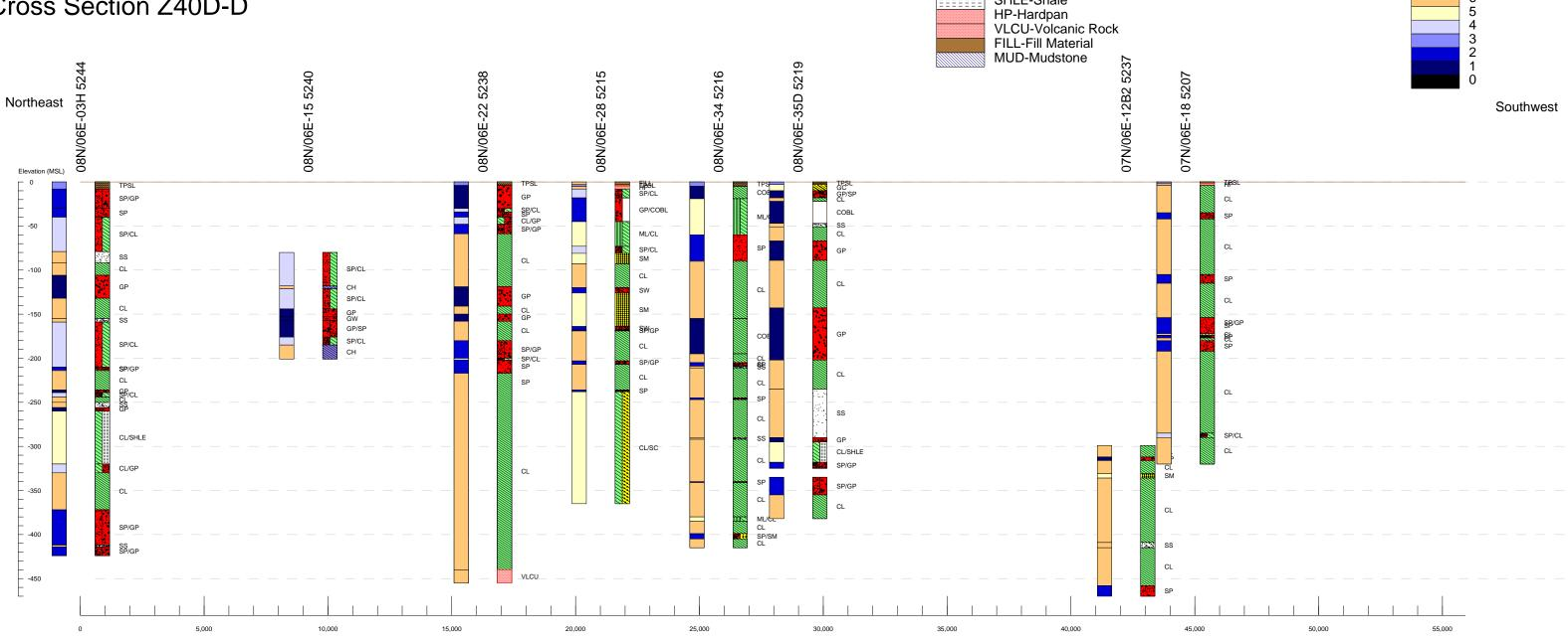
Legend MH 1 COBL-Cobble COBL-Cobble GP-Poorly graded gravel GW-Well-graded fine to coarse gravel SP-Poorly-graded sand SW-Well-graded sand fine to coarse sand GC-Gravel with fines clayey gravel SM-Sand with fines silty sand SC-Sand with fines clayey sand ML-Inorganic silt ..... ML-Inorganic silt ML -Inorganic silt CH-Inorganic clay of high plasticity fat clay CL-Inorganic clay SS-Sandstone SHLE-Shale
