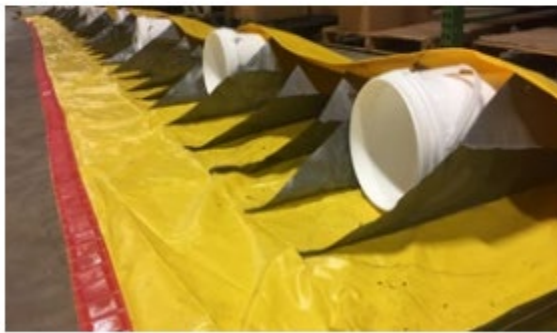
Place objects to raise Water-Gate to dry out, prior to storage
